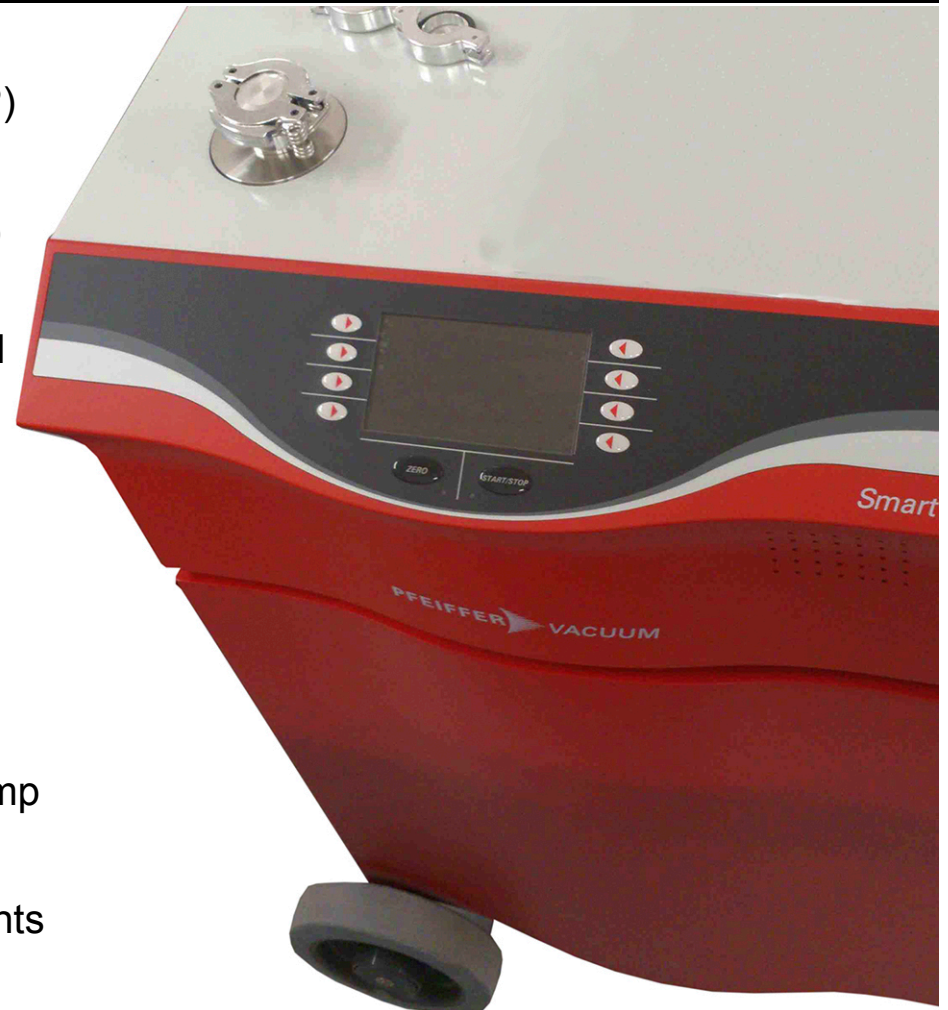
Small helium leak detector delivered as part of VAS test component shipment
