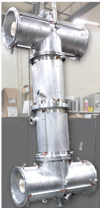
Hybrid Splitter subcomponent for tuning and load-tolerant matching
