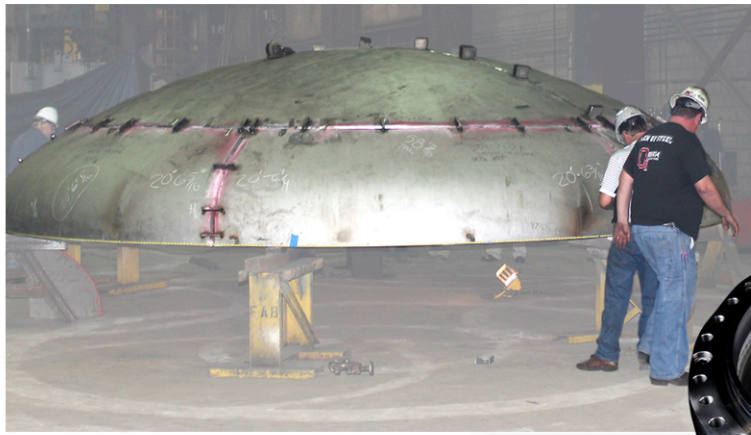
A drain tank head undergoes quality control inspection at ODOM Industries in Milford, Ohio.
