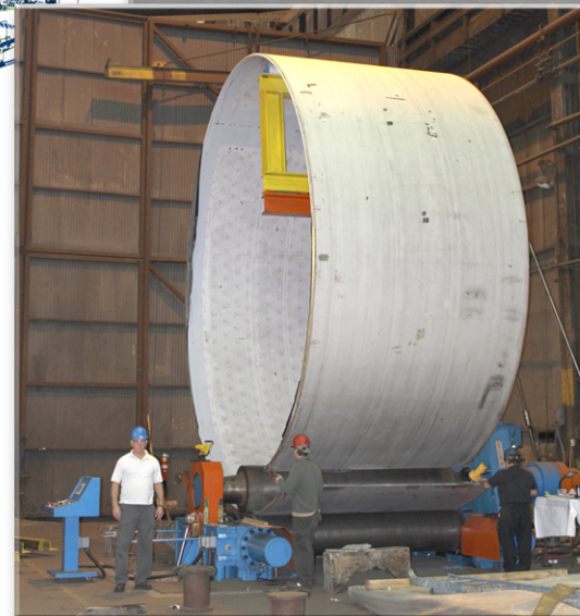
Drain tank rolling is underway at Joseph Oat, Corp. (Camden, NJ)
