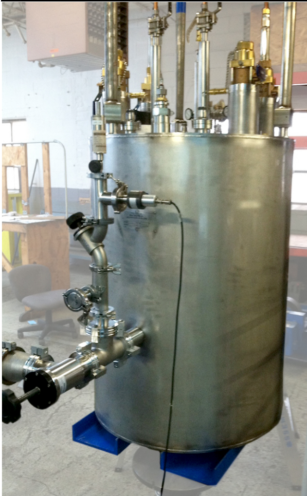
CVC cryogenic valve box Photo: US ITER
