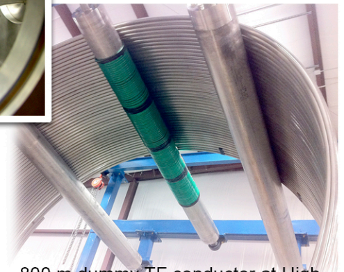
800 m dummy TF conductor at High Performance Magnetics, Tallahassee, Florida.
