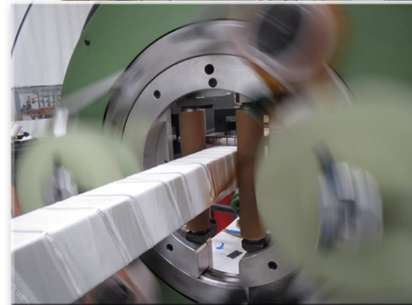
Machine wrapping of conductor bars by Ridgway Machines (Leicester, UK) Photo: General Atomics (San Diego, CA)
