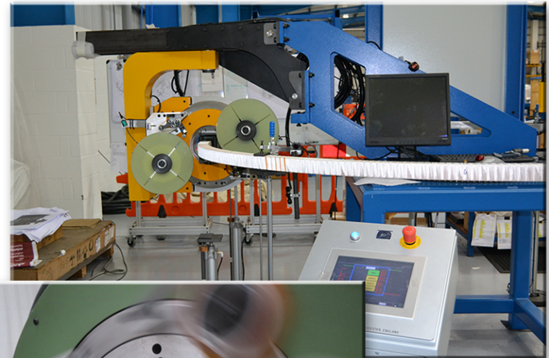
Prototype automated wrapping head Ridgway Machines (Leicester, UK) Photo: General Atomics (San Diego, CA)
