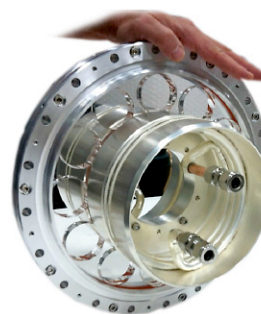
Line and elbow sections with quartz and alumina insulators
