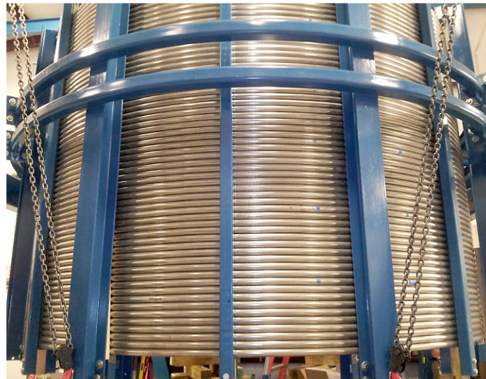
800 m dummy conductor at High Performance Magnetics (Tallahassee, FL)
